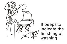
When the washing is finished, the three indicators of "wash" "rinse" "spin" are all on. The power will be switched off automatically about 10 minutes after the finishing of the washing
